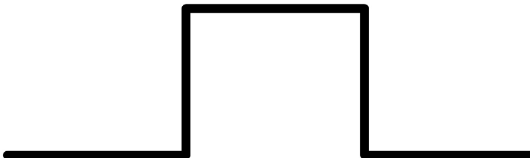
Figure 1: The +110V move up and move down signals are controlled the same way
